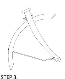
Finish assembly. Make sure there is no fender interference when the tire rotating.
