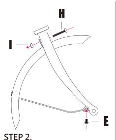
Insert the front fender (A) into the fork and using the provided hardware (H & I) tighten.
